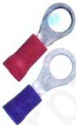
561072 Ring terminal Ring diameter 5mm suitable for 2.5-3mm wire 561078 Ring terminal Ring diameter 5mm suitable for 4mm wire
