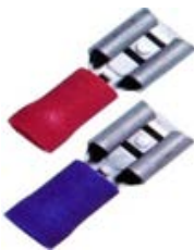
561044 Female blade terminal connector Fully insulated suitable for 4mm wire
