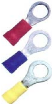
561074 Ring terminal Ring diameter 6.3mm suitable for 2.5-3mm wire 561080 Ring terminal Ring diameter 6.3mm suitable for 4mm wire 561090 Ring terminal Ring diameter 8.4mm suitable for 5mm wire
